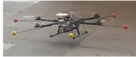
Fig. 1. Our experimental hexacopter unmanned aerial vehicle hovers at low-altitude subjects to severe ground effects. The system employs the Intel Edison computer on-module as its main information processing system. The MAVLink (Micro Air Vehicle communication) protocol interfaces the system to the PixHawk2 Flight Controller Unit (FCU) and the flight stack. Our system has a challenging payload configuration (up to 10 kg take-off weight).
