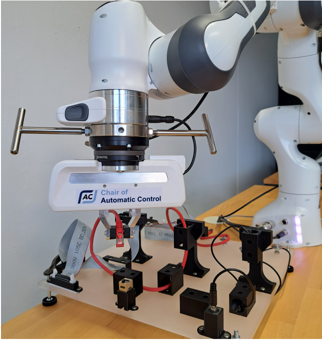
Fig. 2. Experimental setup including the NIST task board #3 [24], a Franka Emika robot equipped with a 6-axis force/torque sensor and a handle bar for kinesthetic demonstration.
