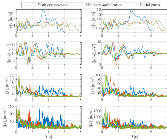
Fig. 8. Experimental results, motion derivatives of minimum jerk (left) and minimum snap (right) trajectories.
