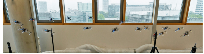
Fig. 1. Composite image of a single drone completing a trajectory generated by the proposed peak-optimization method.
