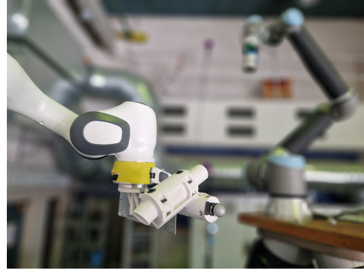
Fig. 6. End effector for Franka robot with hook for connecting the hose. Optical markers are added to the structure for motion tracking. The two bolts on the hose are used as connection points for the magnetic gripper on the UR10e robot manipulator arm.
