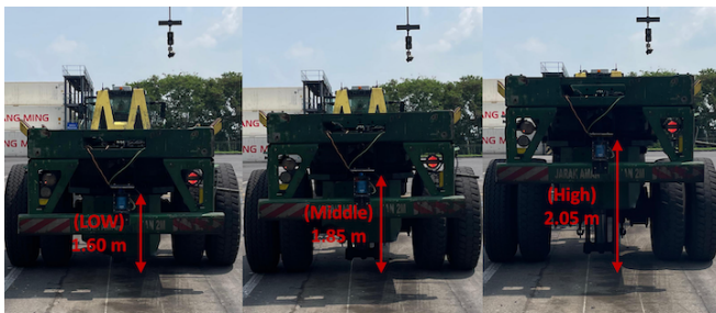
Fig. 3. The LiDAR position on the container truck and its height variability caused by lifting operations.
