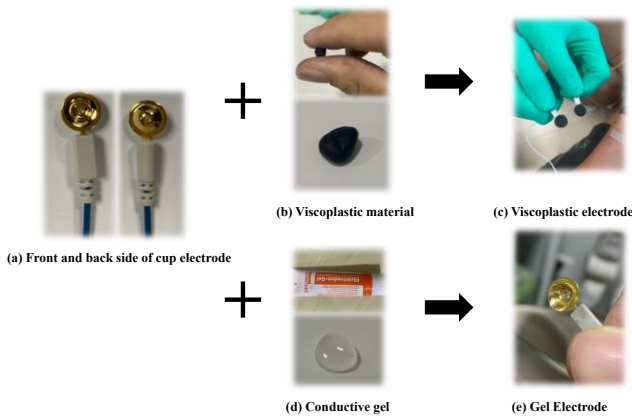
Fig. 1 The photographs of electrodes used in this paper gold standard. First, the impedances of two electrodes group in two adjacent days were tested to investigate the impedance change. Then the physiological signals (ECG and EMG) were obtained by two electrode groups on two adjacent days. Finally, we calculated the difference of the SNR of signals obtained on different days to quantify the performance.
