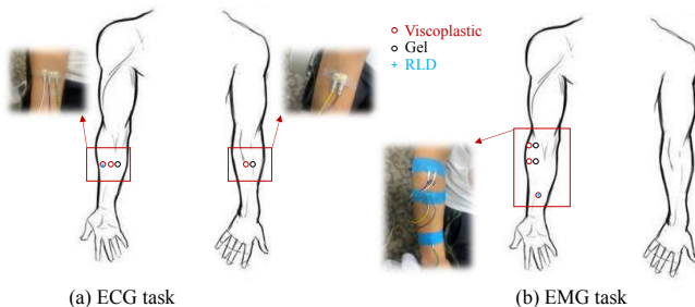
Fig. 2 The positions of the electrodes in (a) ECG and (b) EMG detection tasks
