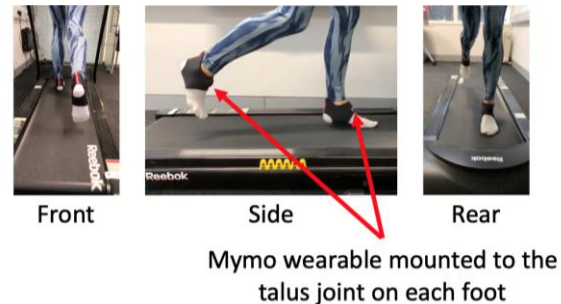
Figure 1: Example of video capture with Mymo sensor from front, side and rear perspectives
