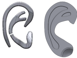
Figure 2. Example of CAD models of the surgical guides created by simplifying the original anatomy.
