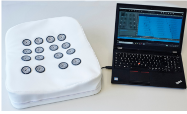
Fig. 1. Multi-channel lung sound recording device.
