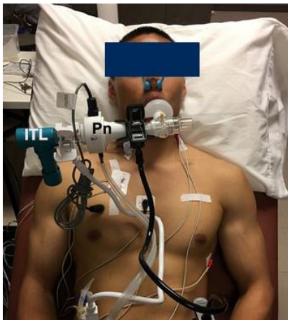
Figure 1. Participant in half-lying breathing in against an inspiratory threshold load imposed by a spring-loaded device (ITL). A pneumotach (Pn) measured inspiratory flow.
