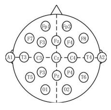
Fig. 1. 10-20 System of EEG electrode placement
