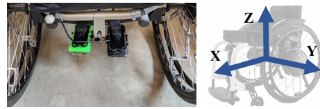
Figure 1. Left: IMU attached to the wheelchair frame; Right: the coordinate system of the IMU
