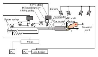
Figure 5. Experimental setup for measuring position P.
