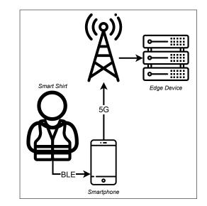
Fig. 5. Envisioned architecture: Powered by the principles of 5G MEC the edge device can be brought into proximity of the smartphone, thereby decreasing latency. Furthermore, data is not sent via the unsafe channel internet, increasing data security. The arrow between cell and edge device is not labeled as there is not de-facto MEC standard, yet.
