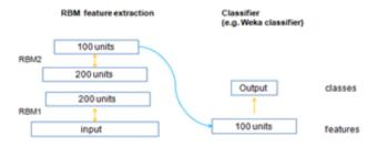
Figure 1. Structure of deep feature extractors: Restricted Boltzman Machine (RBM) with classifier.
