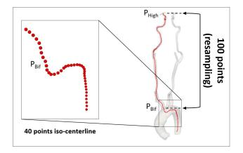
Fig. 2. The resampling interval is chosen such that there are 100 points between  $P_{High}$  and  $P_{Bif}$ . Only 40 points close to  $P_{Bif}$  are kept on resampled centerlines to describe the iso-centerlines: 30 points below  $P_{Bif}$  and 10 above.
