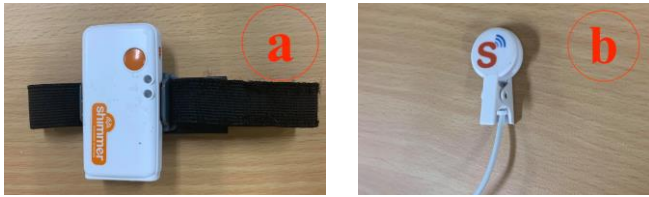
Figure 2. a) Shimmer3™ GSR+ Unit and b) Shimmer3™ PPG-to-HR ear clip
