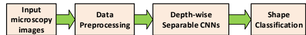
Fig. 2. Suggested stages of shape classification, starting from initial microscopy image to shape classification.
