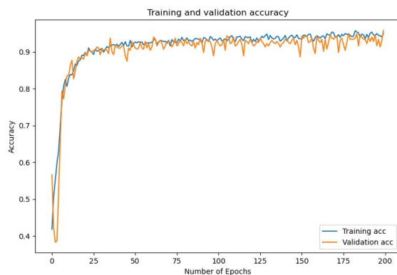
Fig. 5. Validation accuracy using Adam optimizer.
