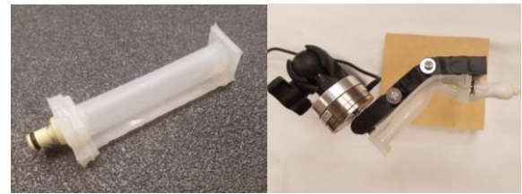
Figure 2. Actuator and Test Fixture. A) Semi-obround actuator with overmolded air connector. B) Actuator test setup with loadcell and force/torque sensor for the dependent variable of the fingertip force resulting from passive resistance to bending the actuator.
