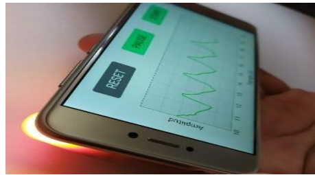
Figure 1. Mobile app developed for smartphones with Android operating system. Example of iPPG signal acquisition.
