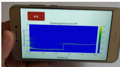
Figure 2. Example of spectrogram and instantaneous RR estimation obtained directly in the developed Android app, for the first two minutes of a maneuver with sudden changes in breathing.
