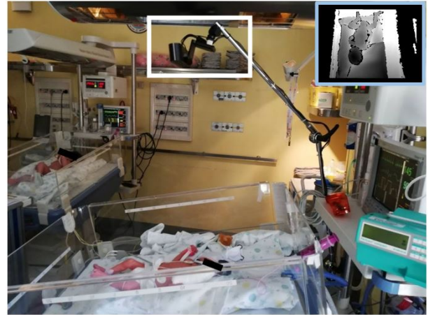
Fig. 1. Depth-image acquisition setup. The depth camera (white square) is positioned \sim 40 cm over the infant's crib, hence leaving the healthcare operators free to move. A sample of depth image is shown on the upper right corner (light-blue square).
