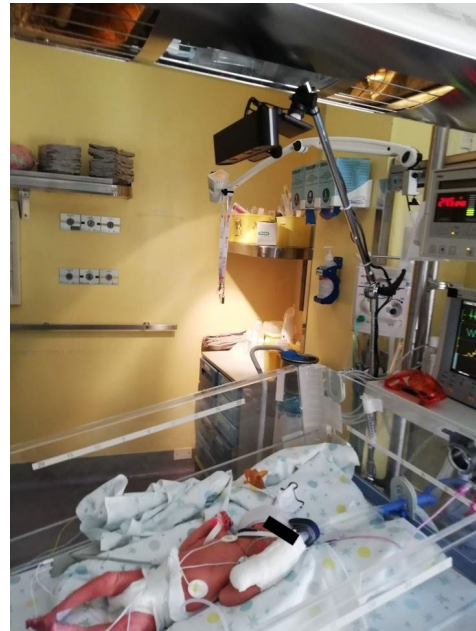
Fig. 1. Depth-image acquisition setup: the RGB-D camera is positioned at approximately 40 cm over the infant's crib.
