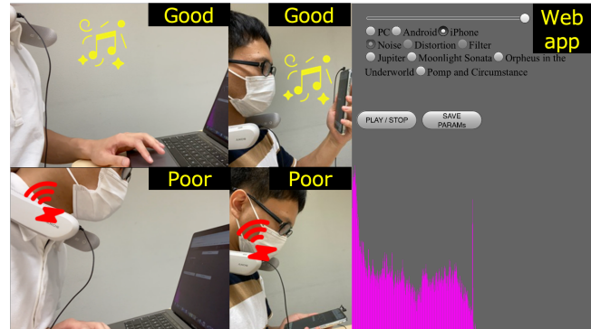
Fig. 1. Posture feedback system with a wearable speaker. Active sensing with ultrasound sent from the wearable speaker to the microphone on their laptop or smartphone estimates the user's posture. When the user's posture becomes poor, they are alerted with auditory feedback from digital audio effects. Audio signal processing is implemented as a web application.
