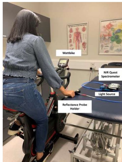
Fig. 1. The measurement set-up of an in-vivo volunteer investigation. The set-up demonstrates an incremental exercise bike study, where lactate concentrations are measured using a commercial portable NIR spectrometer, a light source and a reflectance probe holder, which connects the fiber optic cable to the spectrometer.
