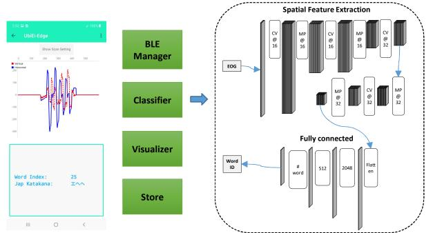
Fig. 2 A system diagram of the proposed UbiEi-Edge mobile platform, which receives the wireless signal via Bluetooth-Low-Energy (BLE), executes the deep learning model, visualizes both the signal and deep learning detection results, and stores the results on the phone. In this study, we will further demonstrate that UbiEi-Edge can enable voice-free communication for ALS patients by decoding eye-written words.
