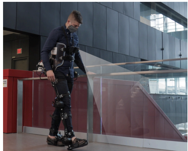
Fig. 1 Photograph of the lead author walking with our robotic lower-limb exoskeleton with environment sensing superimposed.
