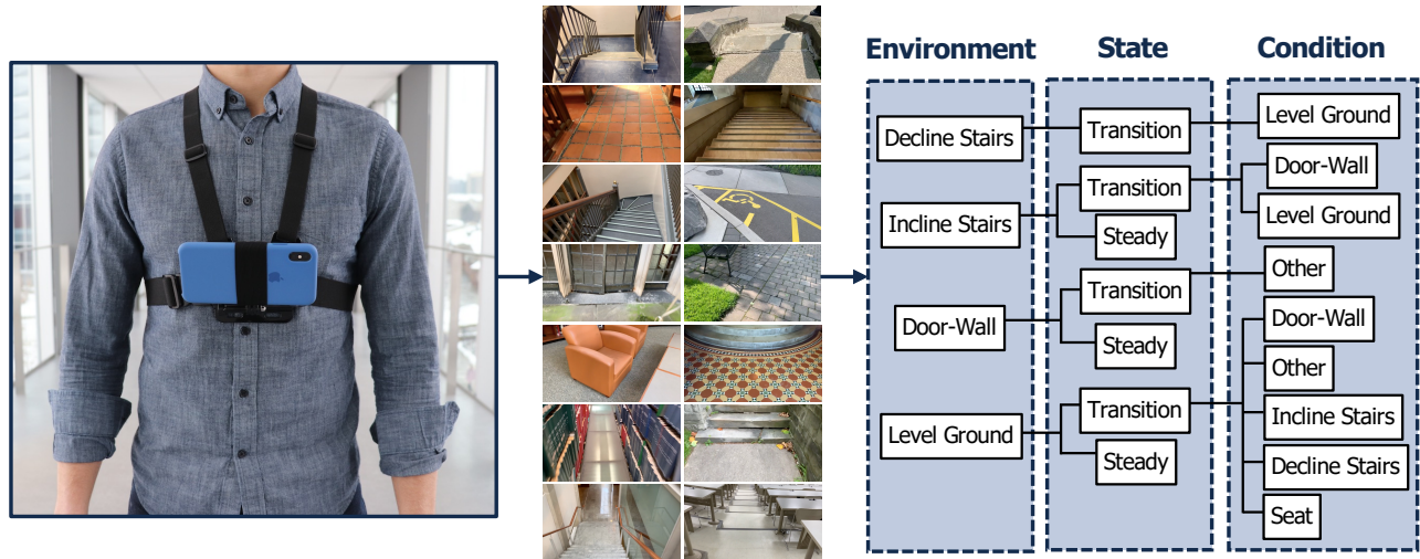
Fig. 2 Review of the ExoNet database, including (left) the wearable camera system used for large-scale data collection; (middle) the high-resolution RGB images of walking environments; and (right) the 12-class hierarchical labelling architecture. For more information, see the original paper [11].
