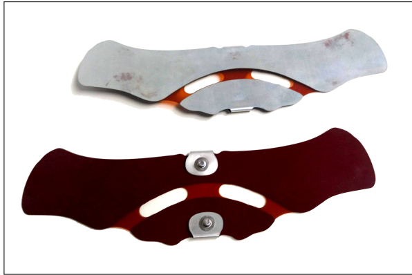
Fig. 3. Custom manufactured flexible electrode pair for ICG with tin [Sn] coating on the front and nonmagnetic steel button terminals on the back.
