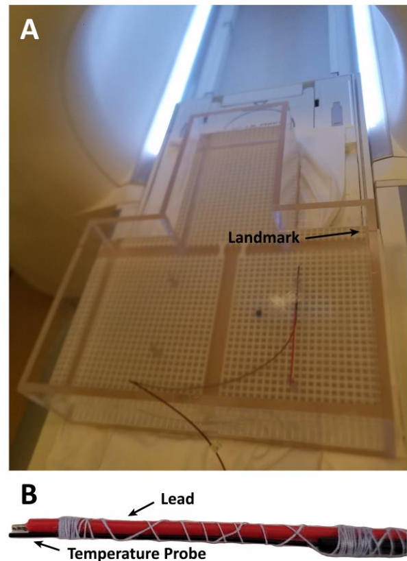
Figure 2. (A) PAA filled phantom with wire and probes in the 1.5 T Aera Scanner. (B) Close up of fluoroptic probe attached to the tip of the generic wire for temperature measurements.
