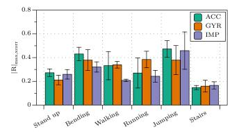
Fig. 5. Median of the maximum cross-correlation coefficient between different sensor types and the ECG-lead I.
