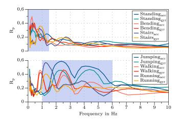
Fig. 4. Median correlation between the ECG and reference sensors depending on the frequency bands.
