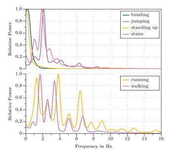
Fig. 2. Frequency spectrum of motion artifacts for different types of movements.
