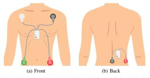
Fig. 1. Electrode and sensor location at the front and the back of the subjects.
