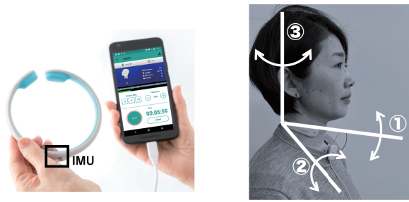
Fig. 2. Left fig.: The neck orientation is shown on the smart-phone's interface in realtime. Right fig.: Measured three neck orientations:①Pitch, ②Roll, and ③Yaw angles.
