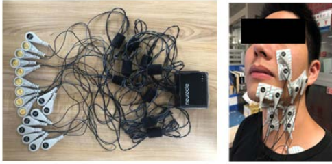
Figure 1. Surface electrode used to collect sEMG signal data and display of electrode positions
