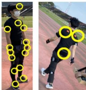
Figure 1. Experimental Setup. The Xsens MTx Awinda were placed at 17 different area on the participant body.
