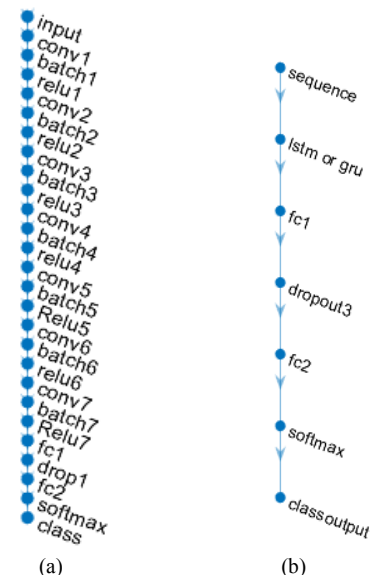
Figure 3: (a) 1D or 2D CNN architecture and (b) LSTM or GRU architecture
