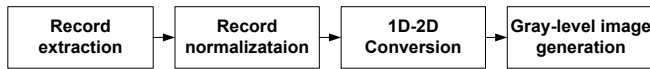
Figure 1. Steps to obtain a 15 x 15 pixels gray-level image of a record with 225 samples extracted around an R-wave peak: record extraction, record normalization, 1D-2D conversion, gray-level image generation.
