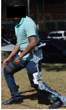
Fig. 1. A subject wearing the exoskeleton ExoTAO.
