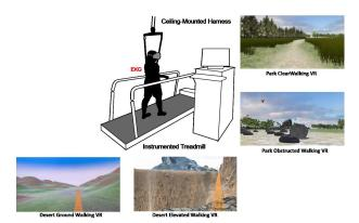
Fig. 1: A depiction of the experimental set up for the VR walking tasks.
