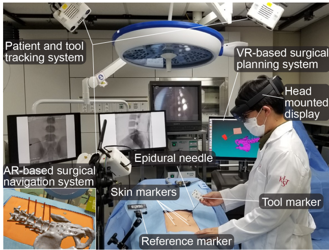
Fig. 1: System overview of the AR-assisted surgical navigation system for epidural needle intervention
