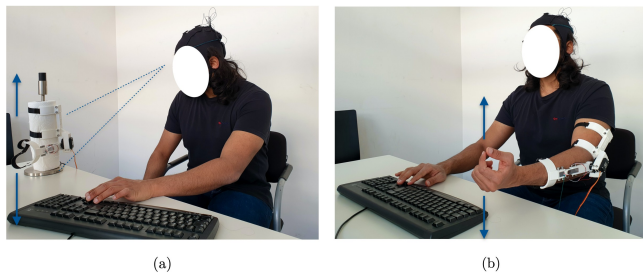
Fig. 2: (a) The observing condition. The user observes the exoskeleton while wearing the EEG headset in the dry-electrode configuration. A visually observed erroneous behavior elicits ErrPs. (b) The wearing condition. The exoskeleton supports flexion or extension, and the user perceives an error if the behavior of the exoskeleton does not match their key-press.
