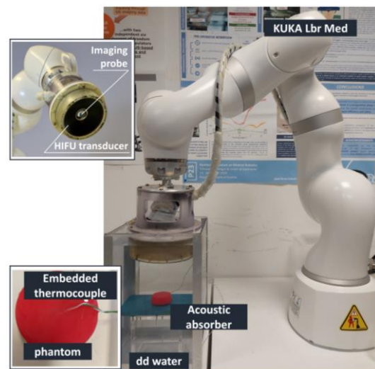
Figure 1. Set-up - The HIFUSK platform is used for delivering the HIFU sonications. The phantom is immersed in a dd-water tank. A thermocouple is embedded in it for measuring temperature during sonications.
