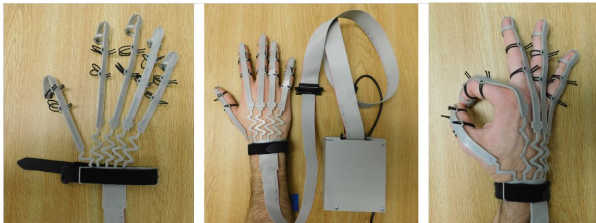
Figure 3. The design of SensoriGlove (Left). Glove connected to DAQ module via ribbon cable and a USB cable that connects it to computer (Center). An American Sign Language (ASL) posture showing the flexions of thumb and index finger and enslaving observed in other fingers (Right).
