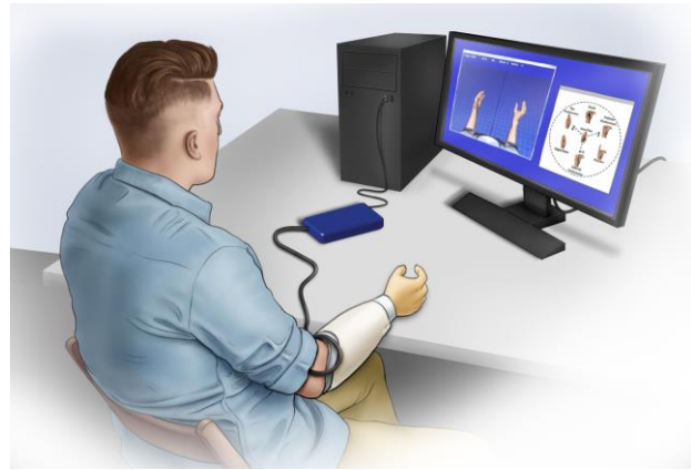
Figure 1– Experimental testing setup including subject with chronically-implanted EMG sensors, data acquisition system, and virtual prosthetic hand interface.
