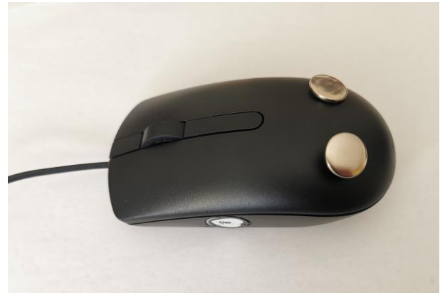
Figure 2. The developed smart mouse with PPG and GSR sensors.
