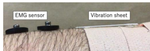
Figure 4. Forearm with EMG sensors and a vibration sheet. of placing it in the socket, which increases the effort to wear the prosthetic hand.
