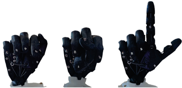
Fig. 1. The adaptive, affordable, open-source TATUM robot hand-wrist system signing the letters A (left), S (center), and L (right).
