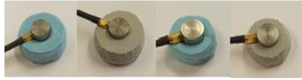
Figure 2. Foam holders left to right: low density / 5.5cm \varnothing , high density / 5.5cm \varnothing , low density / 4.5cm \varnothing , high density / 4.5cm \varnothing .
