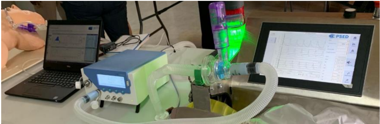
Fig. 2. Bag-valve mechanical ventilator during a functional test, with a IMT Analytics, PF-300 gas flow analyzer as measuring reference.
