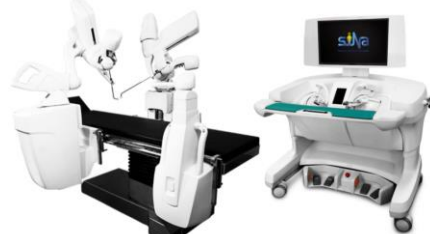
Figure 1. The SINA flex robotic telesurgery system, left: the slave robot, right: the master robot [17].
