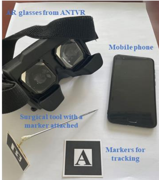
Figure 1. Hardware of the system, showing the mobile phone, the AR glasses, and the tracked surgical tool.
