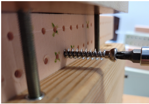
Fig. 2. Example of test sample piece mounted in test rig, miss-drilled holes are marked with a cross. An HB 6.5 screw is pictured carefully aligned and placed against hole ready for testing.
