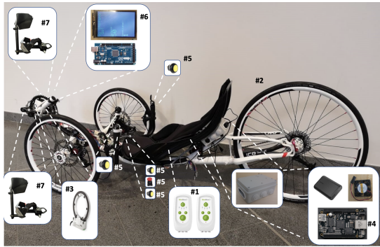
Fig. 1. Experimental setup used in the case study. 1) ReheMove3 stimulators, 2) Trike (Ice VTX), 3) Encoder, 4) Control unit, 5) Push buttons and emergency button, 6) Screen, and 7) AFOs.
