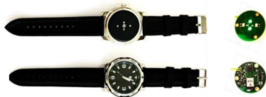
Figure 1, miniaturized wearable wrist PPG sensor.
